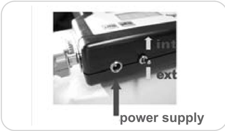
2. Connect the receiver to the PRG\_01 programmer by the cable in equipment (6 poles connector). The external radio receiver must be powered and then disconnect the external power supply
