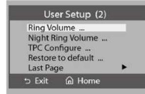
The RING VOLUME option allows to adjust the volume of the played melody in day time (6:00 to 18:00). This monitor allows to set a different volume for calls during night time (18:00 – 6:00) with NIGHT RING VOLUME option.
